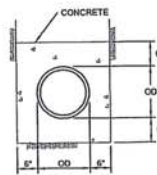
CONCRETE ENCASEMENT DETAIL 2 NOT TO SCALE C002
